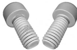
Without (L) / With (R) Scatter|correct screw scan comparison
